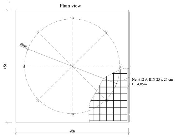
**Reinforcement of foundations plate**
