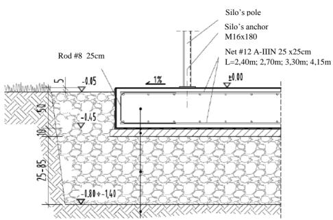
\*Foundation plate of thickeness 50 cm, concrete C20/25 W8. \*Layer of heat-weldable roofing membrane of thickeness at leasts 4 mm. \*Bedding concrete C12/15, thickeness of 10 cm. \*Crushed aggregate, fraction 0-32 mm, volume should be adjusted to the surface conditions. \*Subsoil
