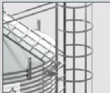
MAIN ENTRANCE LADDER WITH PROTECTION CAGE (SHORT GROUND LADDER AVAILABLE AS OPTION)
